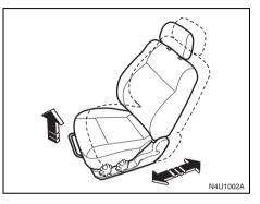
Pull up and hold the bar located under the front of the seat to unlock it. Slide the seat to where you want it and release the bar. Then try to move the seat with your body, to make sure the seat is locked into place.
